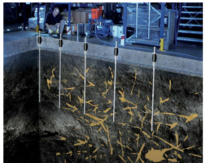
Spread of grout
